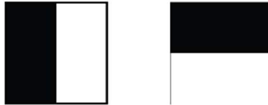
Fig. 9. Haar wavelet filters to compute the responses in x (left) and y direction (right). The dark parts have the weight -1 and the light parts +1 .
