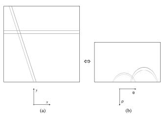
**Figure 4.6.** Straight Line Invariancy: The shape of a straight line after a log-polar transformation is invariant to its position and orientation. (a) Cartesian domain. (b) Log-polar domain.
