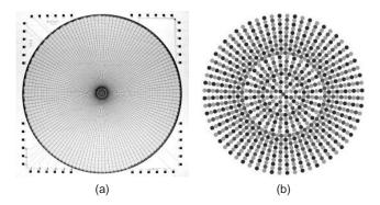
**Figure 3.3.** CMOS 8000 pixel Log-polar sensor: (a) Picture of the 1st version of the CMOS log-polar sensor. (b) Detail of the fovea.
