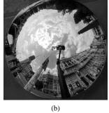
**Figure 5.1.** Panoramic View: (a) Image acquired by an OMNIVIEWS log-polar camera (software simulation). (b) Image acquired by a conventional omnidirectional camera. Note that the image from OMNIVIEWS camera is immediately understandable while the image from a conventional camera requires more that 1.5 million operations to be transformed into something similar with no added advantage.
