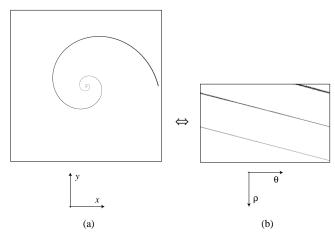
**Figure 4.9.** Logarithmic Spiral: Such a spiral, centered in the origin of the mapping, after a log-polar transformation becomes a straight line. (a) Cartesian domain. (b) Log-polar domain. Please note that in our representation we display the set of points  $\theta_0 + 2k\pi$  all on  $\theta_0$ .
