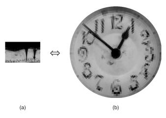
**Figure 3.4.** 8000 pixels CMOS Log-polar sensor simulation: (a) The log-polar transform of the image 3.2a performed by this sensor. (b) The remapped image.
