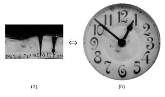
**Figure 3.6.** 33000 pixels CMOS Log-polar sensor simulation: (a) The log-polar transform of the image 3.2a performed by this sensor. (b) The remapped image. Although the remapped images are not in scale, the log-polar ones are in scale between them.
