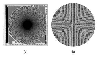
**Figure 3.5.** CMOS 33000 pixel Log-polar sensor: (a) Picture of the 2nd version of the CMOS log-polar sensor. (b) Detail of the fovea.
