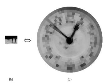
**Figure 3.2.** 2000 pixels CCD Log-polar Sensor Simulation: (a) A standard cartesian image. (b) Its log-polar transform performed by this sensor. (c) The remapped image. Please note that in this figure, and in the next Figs. 3.4 and 3.6, the log-polar image and its transform are not in scale. In all these images the fovea is not displayed.
