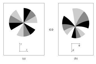
**Figure 4.1.** Angle Preservation: The angles are locally preserved after a log-polar Transformation. (a) Cartesian domain. (b) log-polar domain. Please note that both images a and b are particulars, so the origin of the mapping falls outside of the cartesian image.
