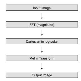
Figure 4.5. The Fourier-Mellin Transform.
