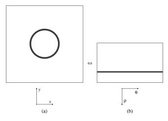
**Figure 4.8.** Circumference Centered in the origin: The shape of a circumference, centered in the origin of the mapping, after a log-polar transformation is a horizontal straight line. (a) Cartesian domain. (b) Log-polar domain.
