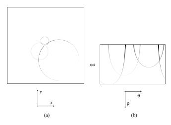
**Figure 4.7.** Circumference Invariancy: The shape of a circumference, passing through the origin of the mapping, after a log-polar transformation is invariant to its position and orientation. (a) Cartesian domain. (b) Log-polar domain.
