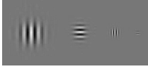
Figure 6. A Gabor function is constructed by multiplying a Gaussian function by sinusoidal function[12]. We use five scales and eight orientations.
