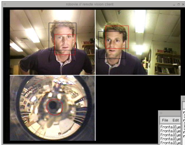
Figure 2. Here are the views that RUBI sees while tracking a face. Top are views from left and right eyes, red box is response from color tracker, black box is response from face-detector. Bottom left is the view of the omni-directional camera.
