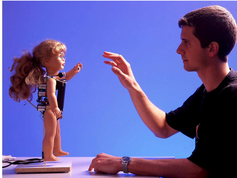
Fig. 1. A PocketPC mounted with a FlyCam Camera tracks the motion of the user and sends commands to the microcontrollers and servos of Robota, so that it can imitate the motion of the head and arms of a user.
