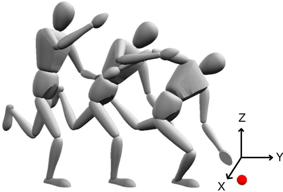
Fig. 3. Hand Control with Joint-Limit Constraints: In this sequence, the robot is commanded to reach a target with its left hand while maintaining self-balance and without violating joint-limit constraints. In the rightmost snapshot, the robot cannot reach farther due to joint limits in the left elbow, right-leg, and upper body.
