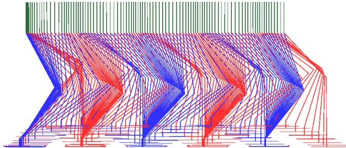
Fig. 16. Stick diagram of the biped walking (spaced 0.03sec ).
