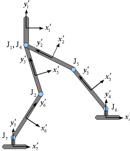
Fig. 2. Model of 6-DOFs biped robot.
