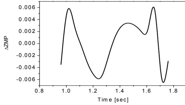
Fig. 7.  $\Delta ZMP$  for the optimized trunk motion,  $x_1(t)$ .
