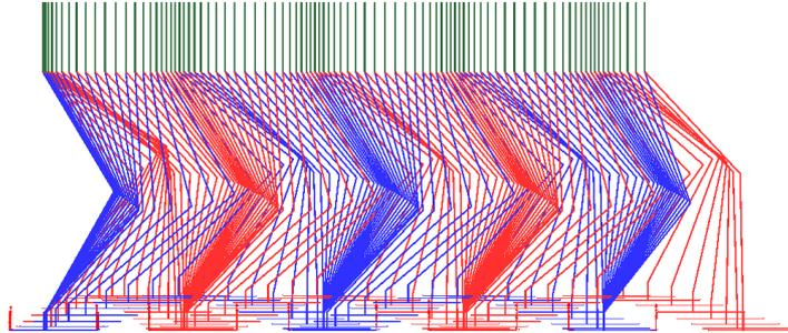
Fig. 15. Stick diagram of the biped walking (spaced 0.04sec ).
