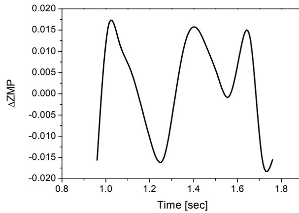
Fig. 12.  $\Delta ZMP$  for the optimized trunk motion,  $x_1(t)$  .
