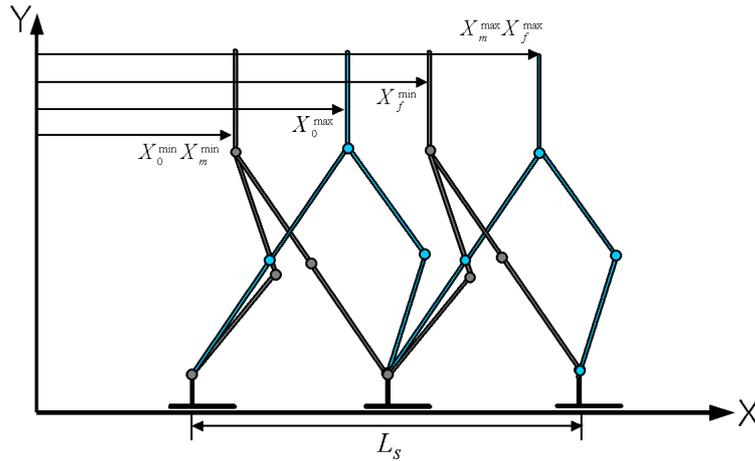
Fig. 4. Kinematic limitations of the biped robot.
