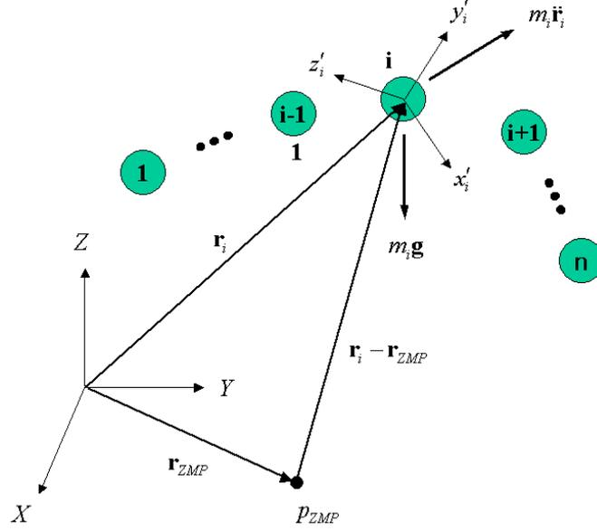
Fig. 1 The reference frame and the ZMP.
