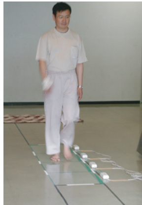
Fig. 3. Pressure Distribution Measurement of Stance Foot
