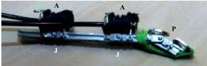
Fig. 2. digit with two fluidic actuators (A) integrated to the joints (J), and one passive joint (P) with return spring.
