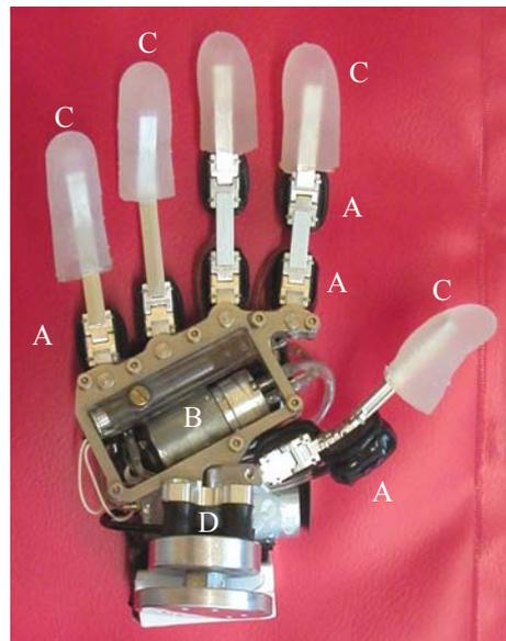
Fig. 3. Humanoid Robot hand with 8 fluidic actuators (A), integrated pressure unit (B), soft finger pads (C) and a passive wrist joint (D)
