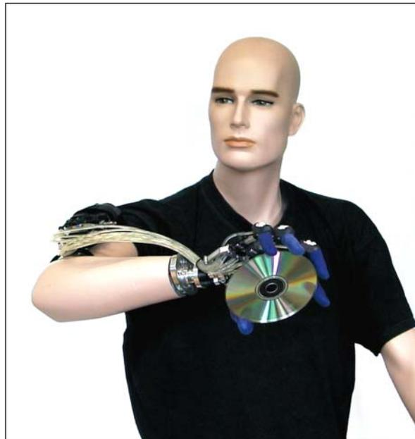
Fig. 4. Manikin wearing a fluidic hand with external pressure unit at the upper arm. The opening span of the hand of 150mm allows for grasping large objects .
