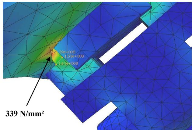
Fig. 7. FEM stress simulation. Detail of the joint connector.
