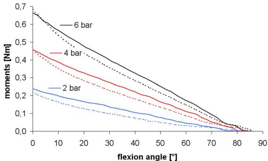
Fig. 5. The moment characteristic of a flexible fluidic actuator at three different filling pressures (2,4,6 bar), (solid lines) and the influence of the spring element (dotted lines).
