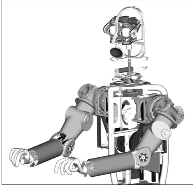
Fig. 1. CAD model of the Humanoid Robot with lightweight humaniform arms and hands. (© MKL, University of Karlsruhe, Germany).
