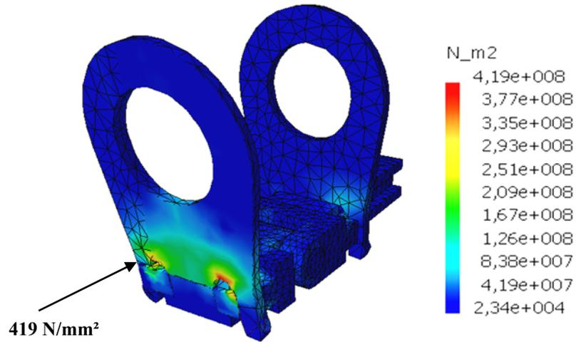
Fig. 6. FEM simulation of stresses on the joint.
