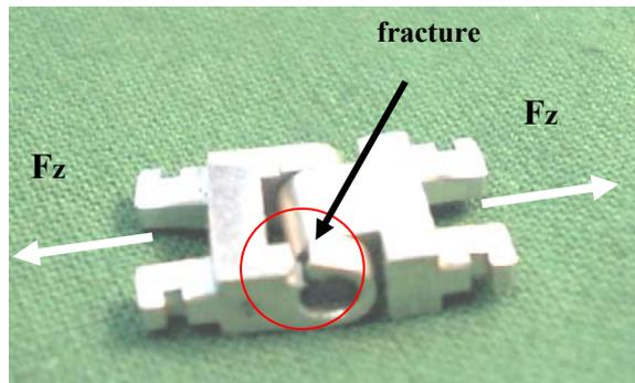
Fig. 9. Fractured joint from tensile testing
