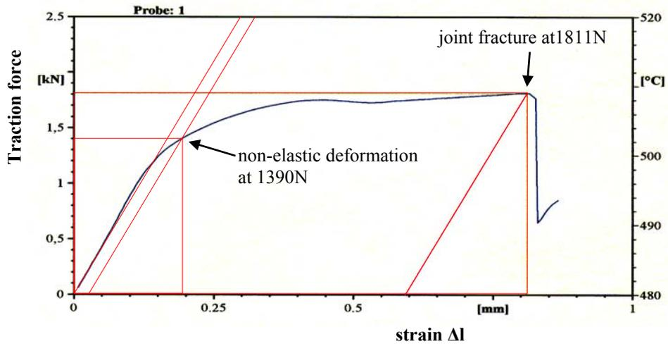
Fig. 8. Stress-strain diagram of a joint.
