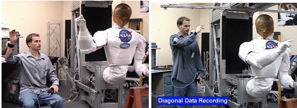
Fig. 1. A human teleoperating of the NASA Robonaut using our IMU-based motion capture system.
