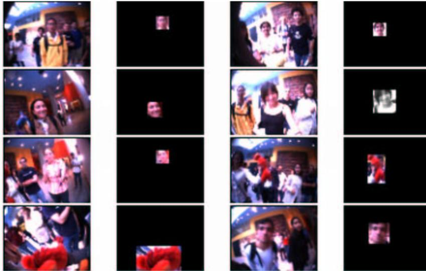
Fig. 10. Examples of the attentional system's output while the robot interacts with multiple people on day 2 of the Phase II experiment. On the first and third columns are the robot's visual input. On the second and fourth columns are the corresponding output of the attention system indicating where the robot should be orienting to and tracking
