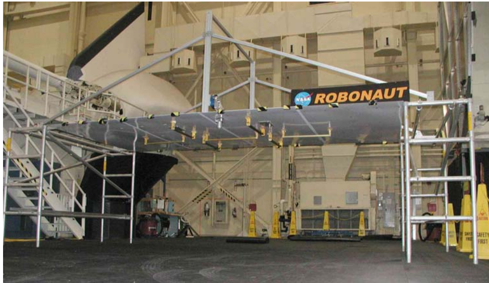
Fig. 9. Planar climbing mockup constructed over air-bearing floor.
