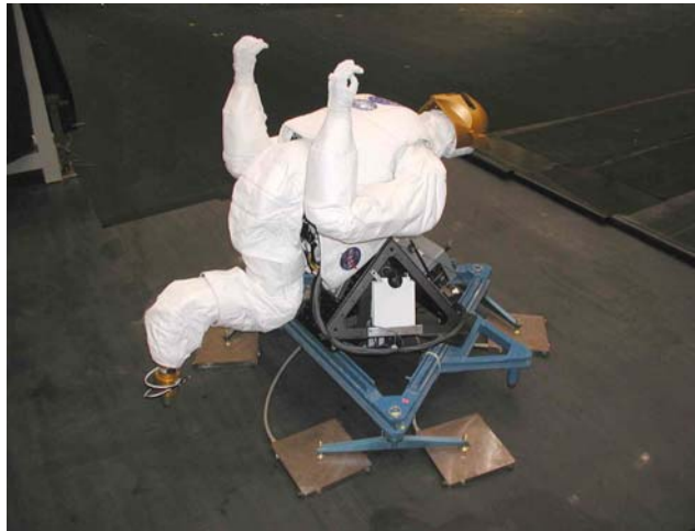
Fig. 8. Robonaut mounted on an air-bearing sled.
