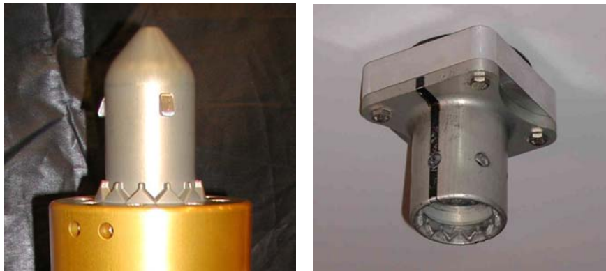
Fig. 11. (left) Latching foot; (right) WIF socket.
