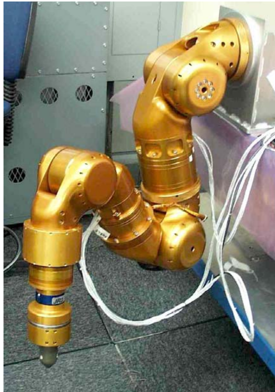
Fig. 7. The first six distal joints and latching foot of the 7 DOF Robonaut zero-g stabilizing leg.
