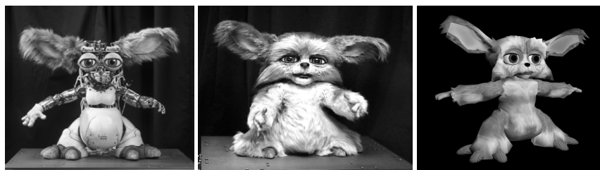
Figure 1: Leonardo is a 65-degree of freedom (DoF) fully embodied humanoid robot that stands approximately 2.5 feet tall. It is designed in collaboration with Stan Winston Studio to be able to express and gesture to people as well as to physically manipulate objects. The left picture shows the robotic structure, the center picture shows the robot when cosmetically finished, the right shows a simulated version of the robot.
