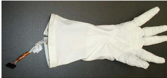
Figure 13: Robonaut tactile glove
