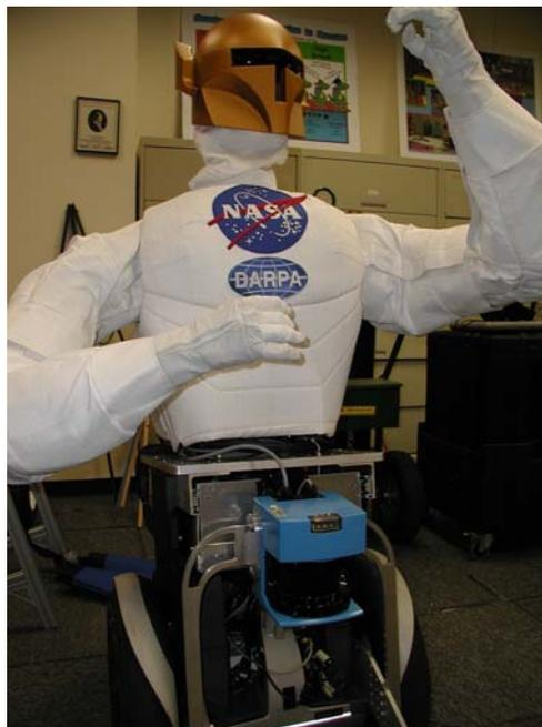
Figure 12: Robonaut with SICK laser
