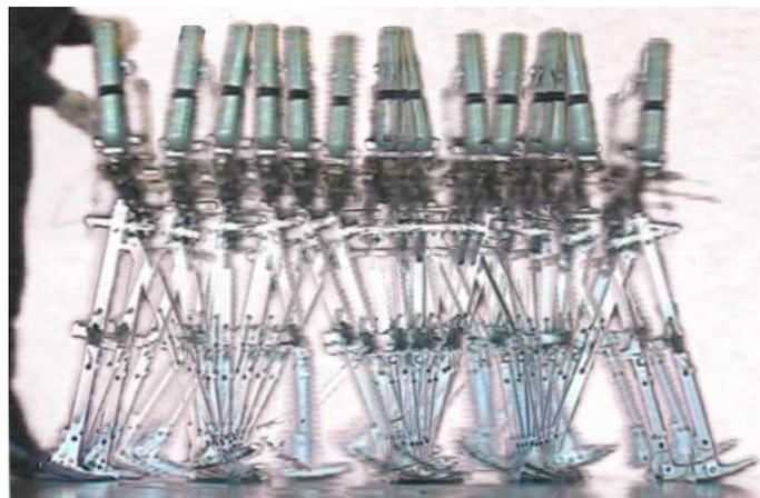
Fig. 10. Video stills illustrating the walking motion after a manual launch.
