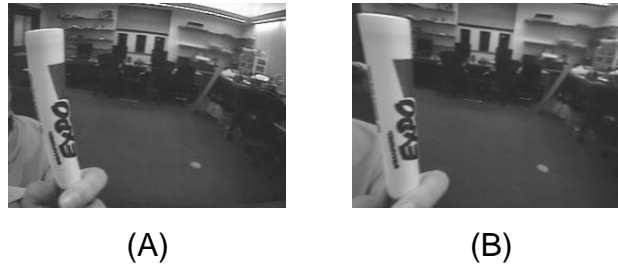
Fig. 3. Original image (A) and image (B) corrected for radial distortion through Eq. (1)
