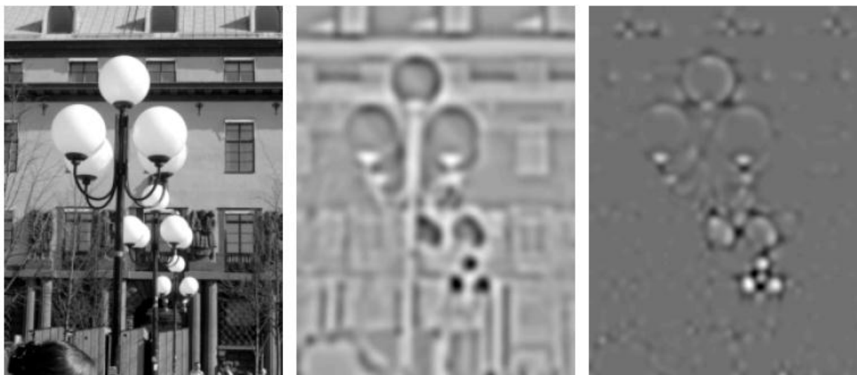
Figure 4: Differential descriptors for blob detection/interest point detection: (left) A grey-level image of size 210 \times 280 pixels. (middle) The Laplacian \nabla^2 L computed at t = 16 . (right) The determinant of the Hessian \det \mathcal{H}L computed at t = 16 .
