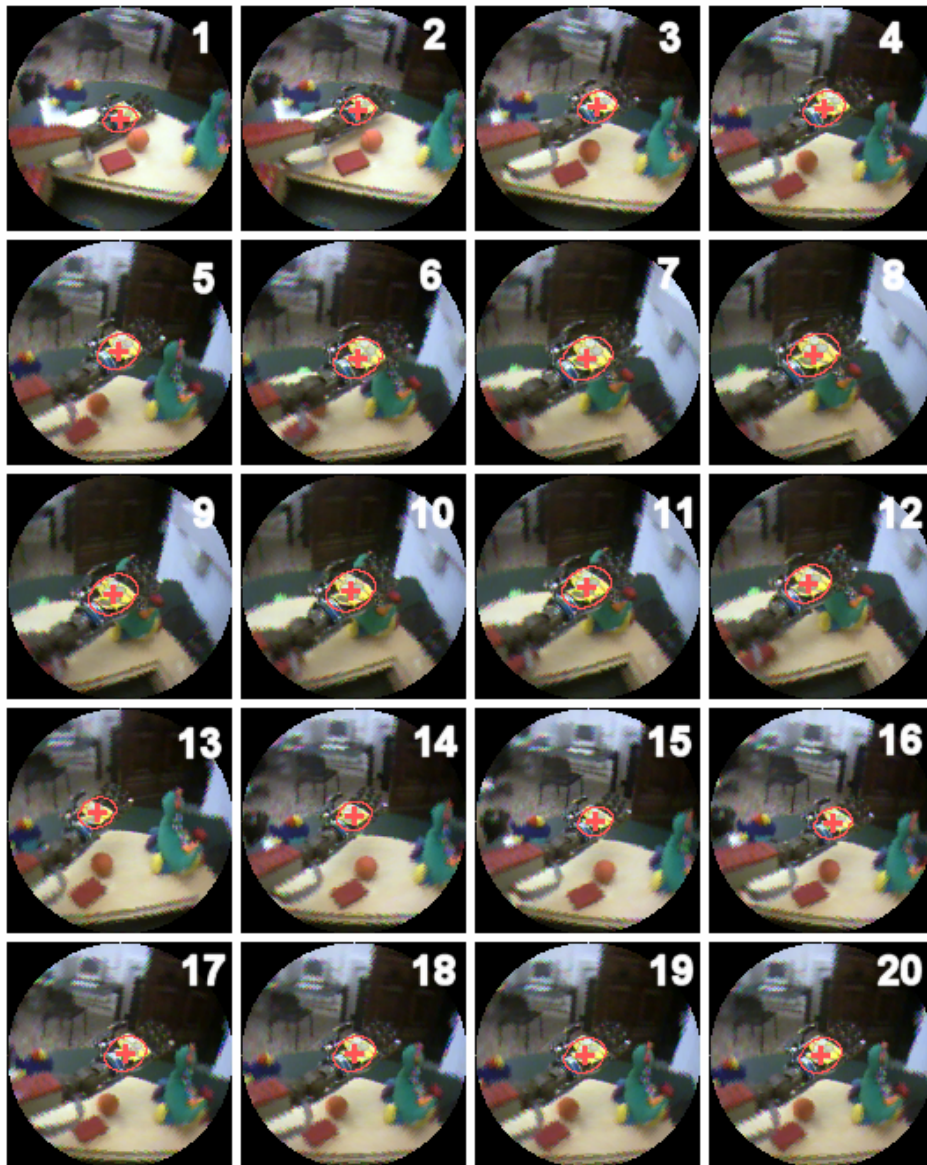
Figure 5.14. Hand localization (1). Frames from a 20 second sequence of the robot tracking the hand (each frame is taken at 1 second interval). The cross represents the position of the hand estimated from the arm posture, the ellipse plots its approximate shape; the gaze of the robot is controlled to maintain fixation on the cross.
