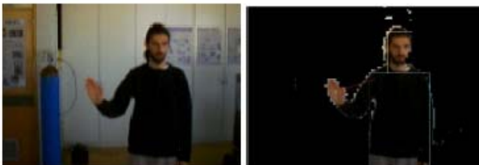
Figure 23: Vision system. Left: original image. Right: background segmentation with human (the frame corresponds to the template matching) and hand detection.
