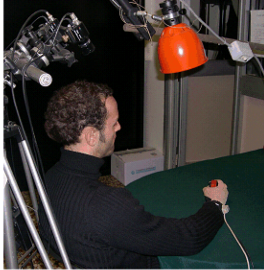
Figure 8: The recording setup. The user wears the cyber glove and reaches for an object. Cameras in this image are placed behind the person and see a good portion of the table. The visual environment for the experiments was well controlled (e.g. illumination) and the background was made uniform in color.
