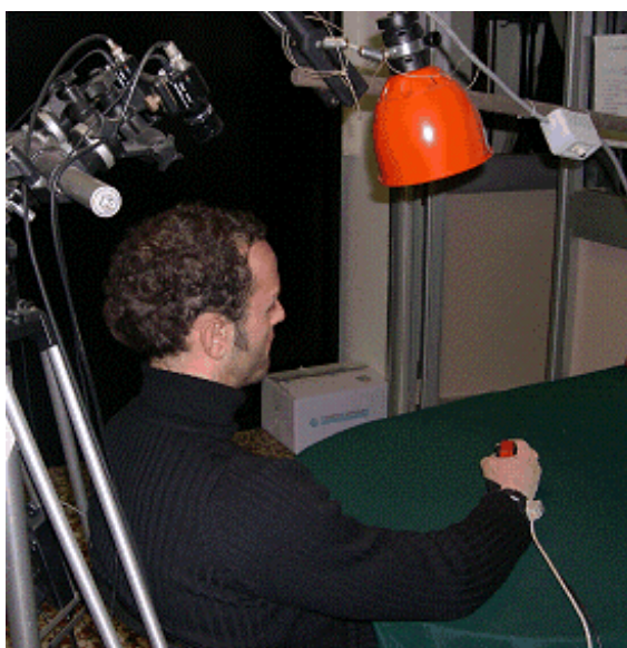
Figure 8: The recording setup. The user wears the cyber glove and reaches for an object. Cameras in this image are places behind the person and see a good portion of the table. The
