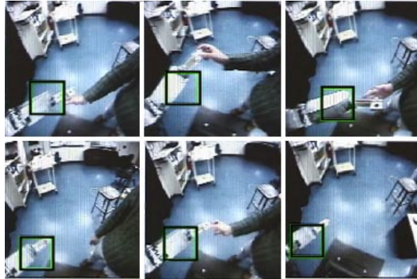
Figure 7. Predicting the location of the arm in the image as the head and arm change position. The rectangle represents the predicted position of the arm using the map learned during a twenty-minute training run. The predicted position just needs to be sufficiently accurate to initialise a visual search for the exact position of the end-effector.
