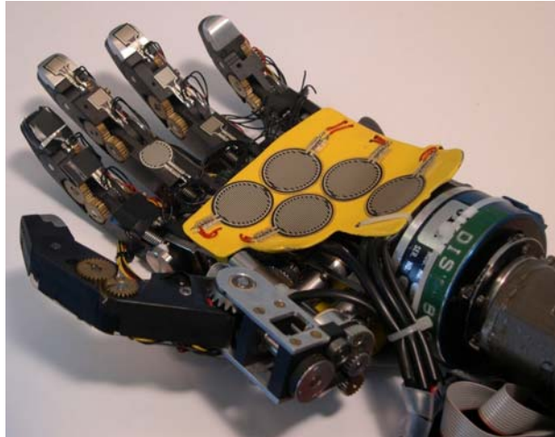
Figure 6 Tactile sensors. 17 Sensors have been placed: five in the palm, three on each finger apart the little finger. In this picture the sensors in the thumb are hidden. The short blue cylinder that links the PUMA wrist to the hand is the J3R force sensor.
