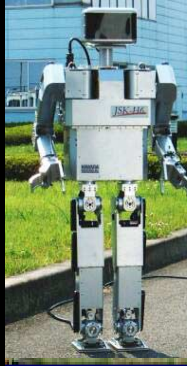
H-7 design and construction S. Kagami, Univ. of Tokyo
