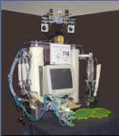
The service robot ISAC pneumatic actuators by Alan Peters Vanderbilt University
