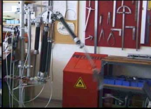
Humanoid robot pneumatic actuators by Rudolf Bannasch, TU Berlin
