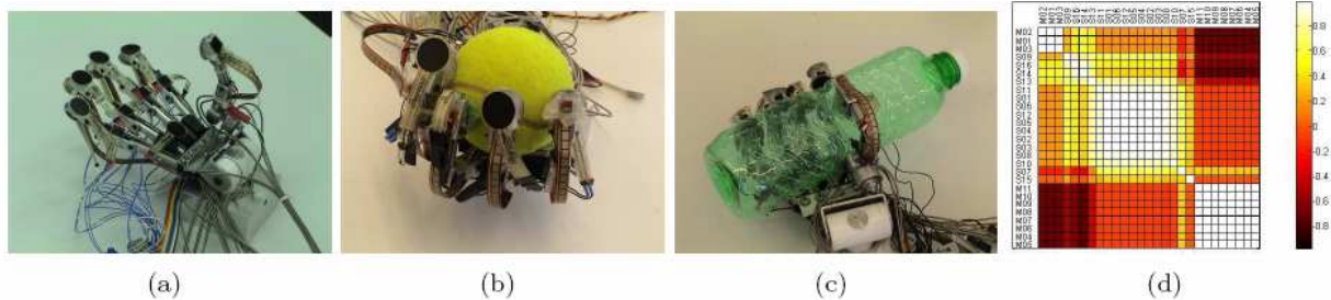
Figure 16: Tendon driven robot hand in (a), (b) and (c) grasping different objects. (d) correlation matrix obtained from the pair-wise correlation of the bending sensors, pressure sensors, and motor encoders for one particular experimental run.
