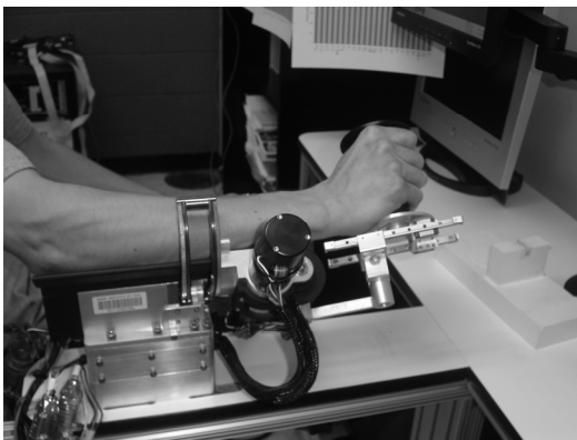
Fig. 1. Photograph of the novel 3-DOF Wrist Robot.
