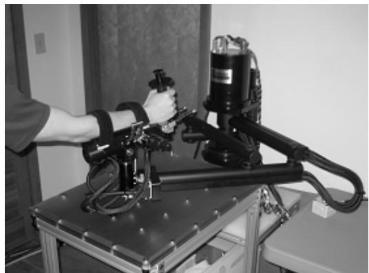
Fig. 3. Robot with 5 active and 2 passive dof.
