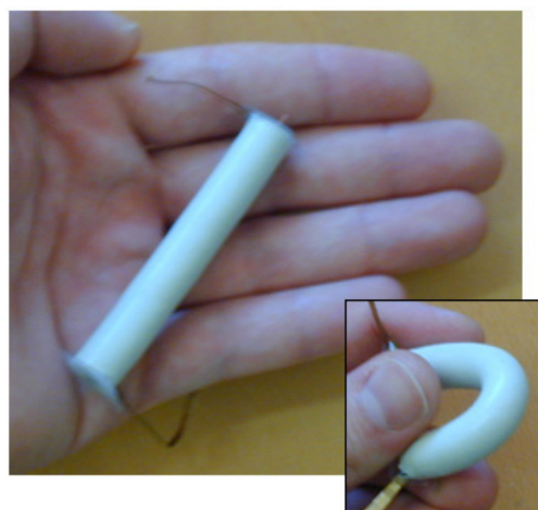
Figure 8. Pictures of a prototype of the new type of dielectric elastomer actuator.
