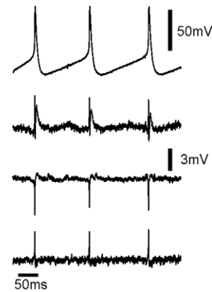
Fig. 10. Simultaneous records at different positions of the same excited snail neuron. Top trace: intracellular voltage with three action potentials. Lower traces: records of three sensor transistors of CMOS chip with different waveforms.
