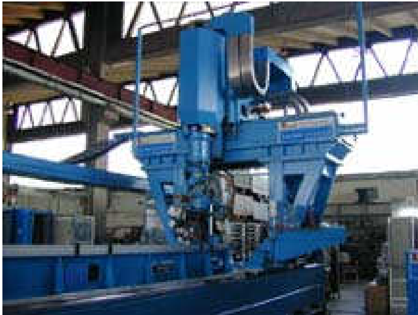
LOONG gantry robot developed to weld train frames
